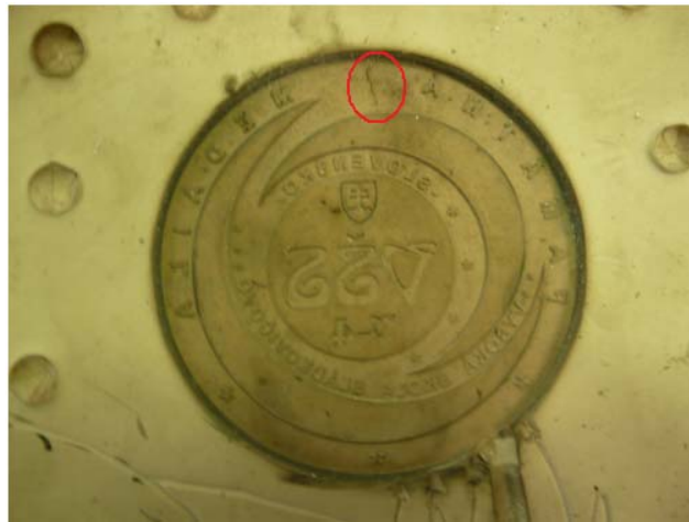
Fig. 1. The crack in the mould's cavity caused by thermal loading
