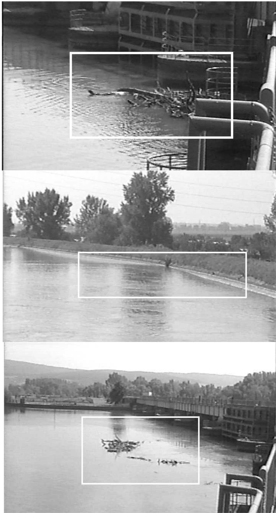
Fig.5 Cleaning trails of screens using water wave
