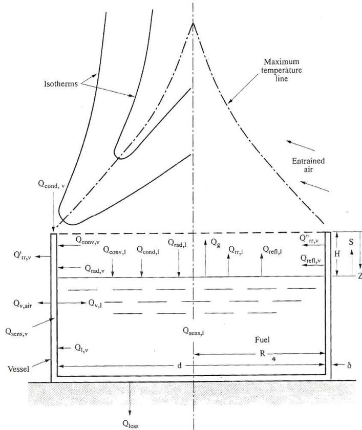
**Fig. 2 Heat transfer in the vessel and liquid [3]**
