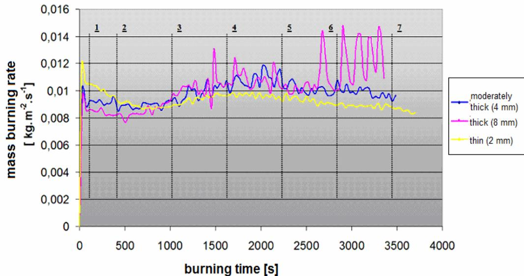
*Fig. 5 Ethanol mass burning rate in dependence on burning time*
