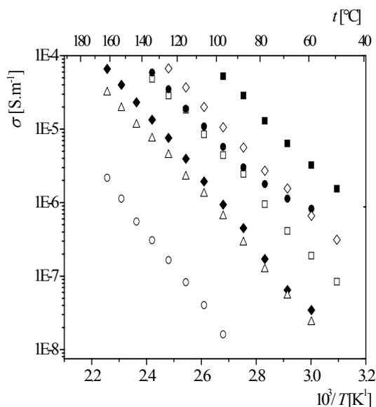
**Fig. 4** The temperature dependence of conductivity for selected glass samples containing praseodymium, holmium and erbium in the form of metal (K) or oxide (O) and without rare earth impurities
