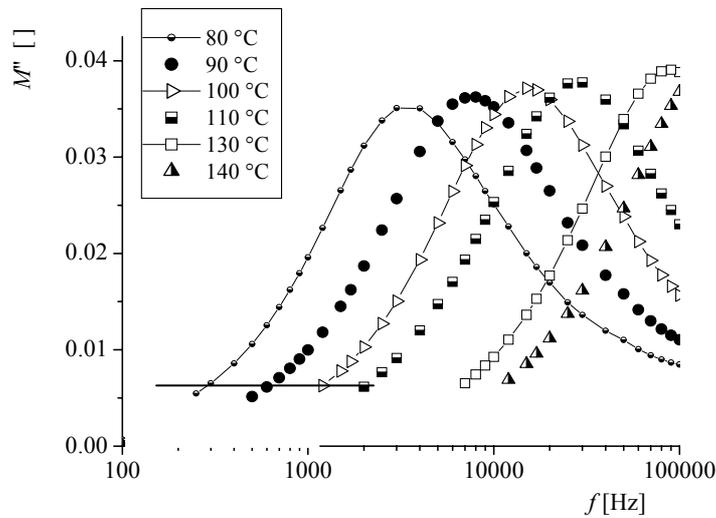
**Fig. 3** Frequency dependences of imaginary complex electrical module ( $M''$  vs.  $f$ ) at different temperatures for  $Ge_{20}Se_{65}Te_{15}+2000$  wt. ppm Ho (as metal) glass
