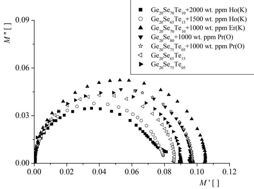
**Fig. 1** Dependence of complex electrical modules ( $M''$  vs.  $M'$ ) measured at 70 °C for samples of glass containing praseodymium, holmium, erbium in the form of metal (K) or oxide (O) and without rare earth impurities.
