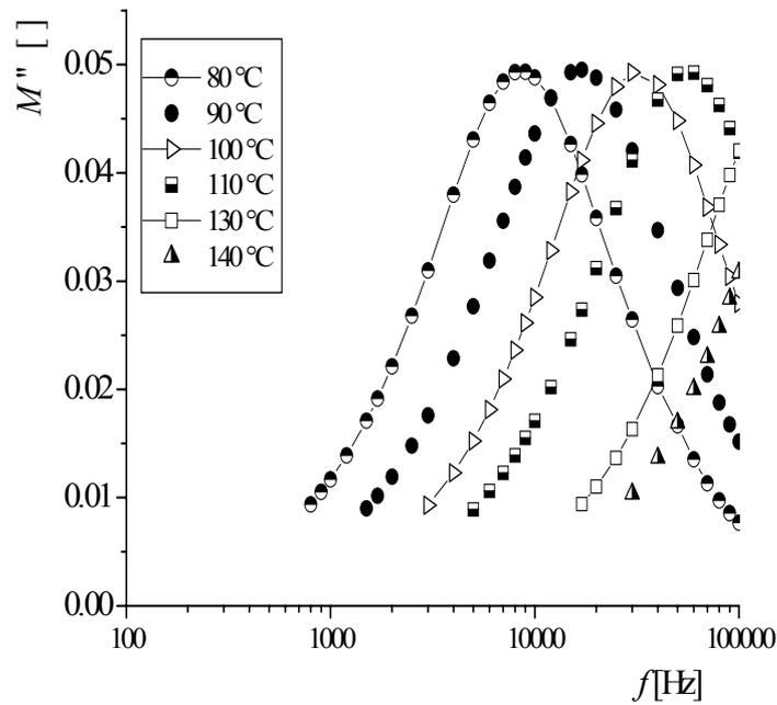
**Fig. 2** Frequency dependences of imaginary complex electrical module ( $M''$  vs.  $f$ ) at different temperatures for  $Ge_{20}Se_{65}Te_{15}+1000$  wt. ppm Ho (as metal) glass
