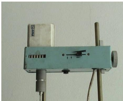
*Fig. 10 Engine of stirring*
