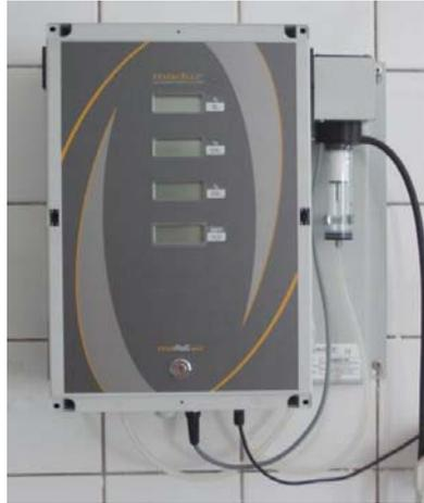
**Fig. 12** Biogas analyzer MaMoS 400
