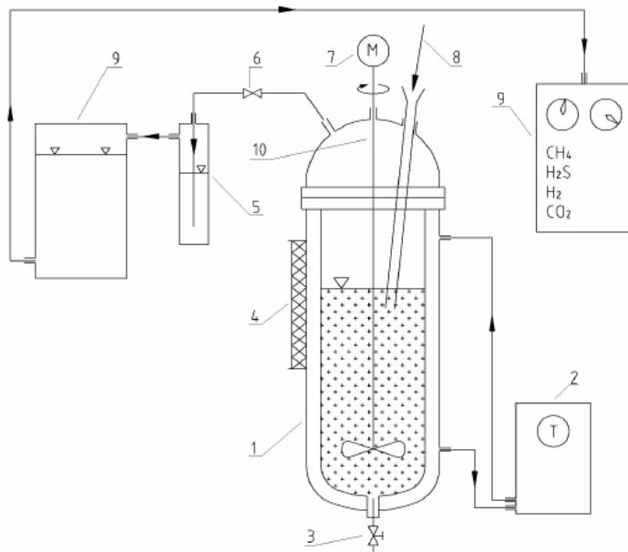
1-Bioreactor, 2-Thermostat, 3-Feedstock outlet, 4-Isolation, 5-Washer,
