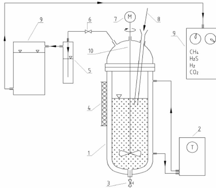
1-Bioreactor, 2-Thermostat, 3-Feedstock outlet, 4-Isolation, 5-Washer, 6- Permeable valve, 7-Engine, 8-Feeding, 9-Biogas analyzer, 10-Stirrer
