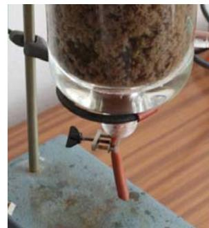
*Fig. 4 Bioreactor outlet*
