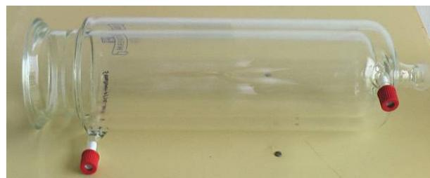
*Fig. 5 Bioreactor, volume 3000 ml*
