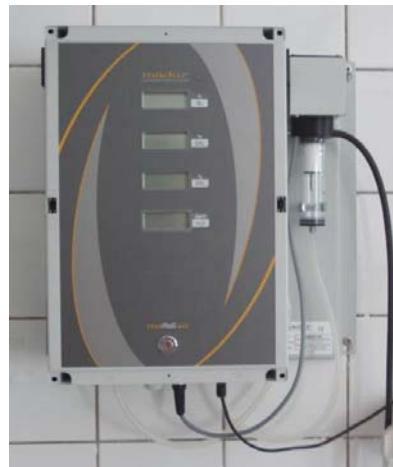
**Fig. 12 Biogas analyzer MaMoS 400**
