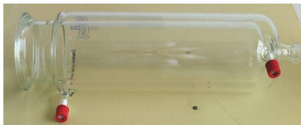
*Fig. 5 Bioreactor, volume 3000 ml*
