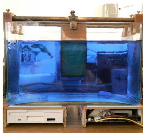
**Fig. 2** Experimental electrolyser
