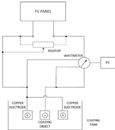
**Fig. 1** Scheme of experimental set with energy obtained from PV panel
