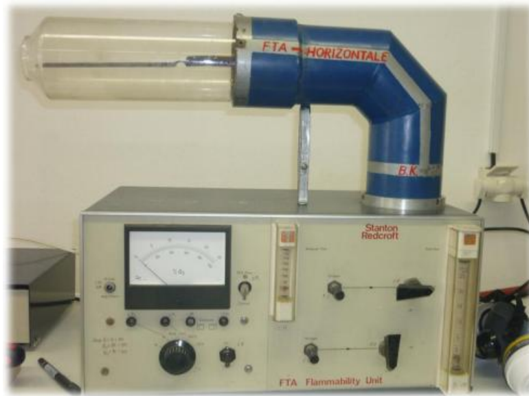
Fig. 6 Photo of the used FTA Flammability apparatus
