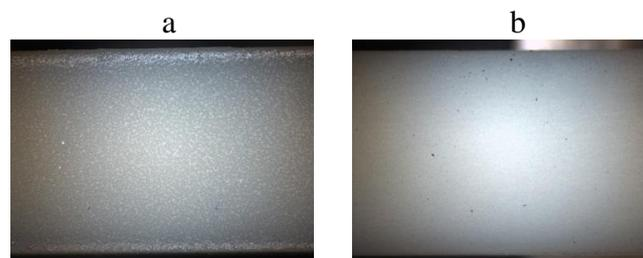
**Fig. 4** Particle dispersion of the PTFE-particles in the matrix:
