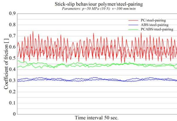
**Fig. 1** Friction behaviour of various amorphous thermoplastics
