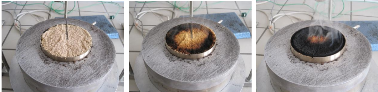
Fig. 2 Carbonization of dust sample during the testing
