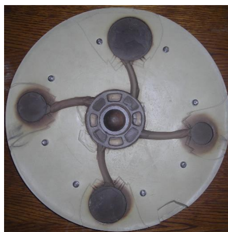
Fig. 1 Silicone mold used for thermal stress measurement
