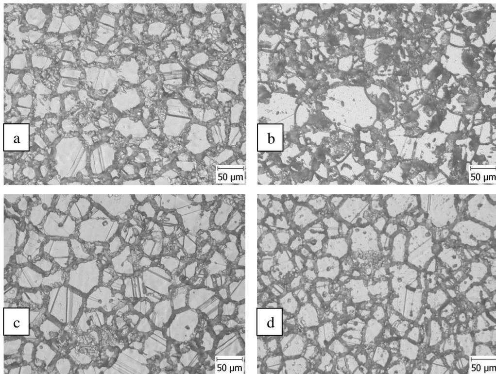
**Fig. 2** Microstructure of steel P560 after corrosion tests under conditions: a) 750 °C/30min.; b) 750 °C/10 hrs.; c) 900 °C/30 min.; d) 900 °C/10 hrs.
