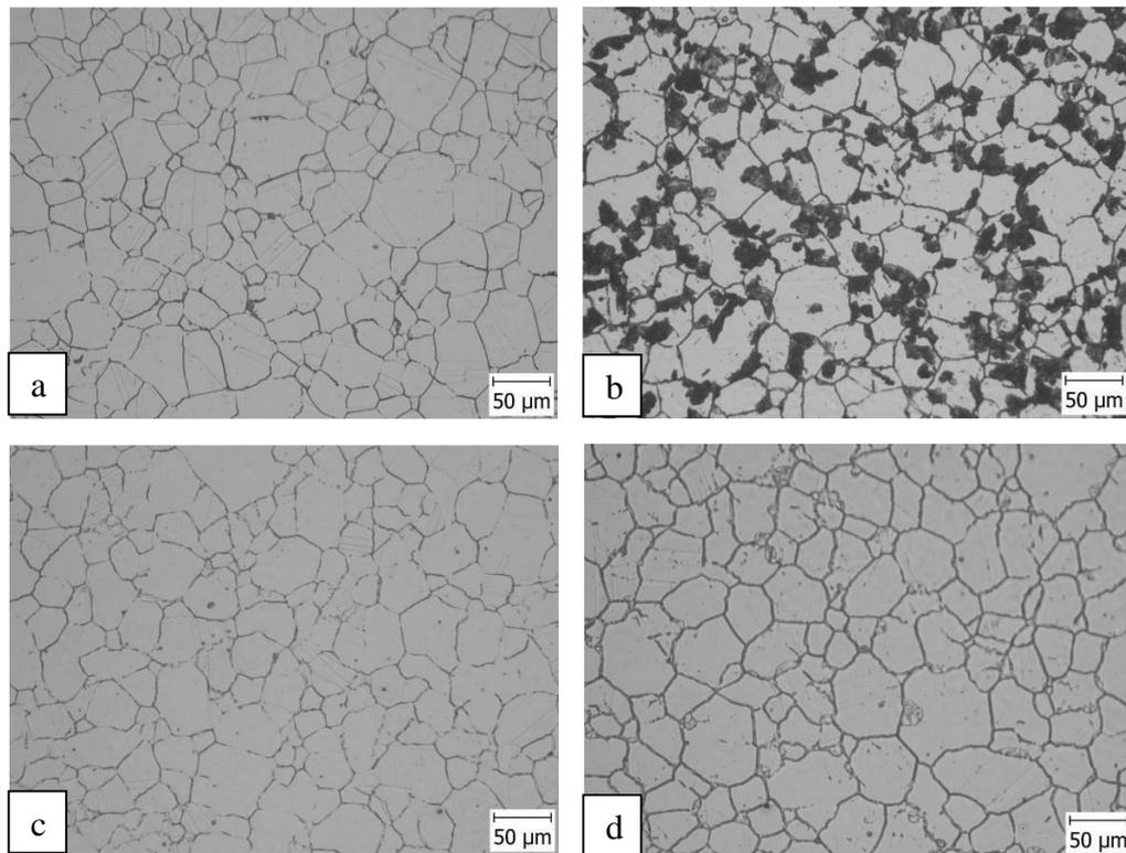
**Fig. 1** Microstructure of the steel after isothermal annealing under conditions a)  $750\text{ }^{\circ}\text{C}/30\text{ min}$ ; b)  $750\text{ }^{\circ}\text{C}/10\text{ hrs.}$ ; c)  $900\text{ }^{\circ}\text{C}/30\text{ min.}$ ; d)  $900\text{ }^{\circ}\text{C}/10\text{ hrs.}$
