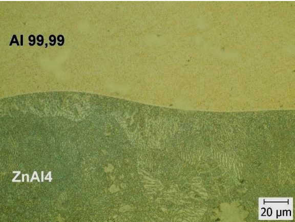
Fig. 4 Microstructure of Al/ZnAl4 soldered joint
