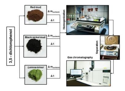
Fig. 1 Working procedure scheme of 3,5-dichlorophenol reduction
