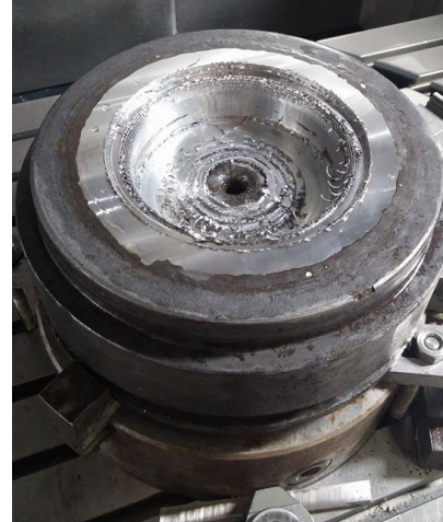
Fig. 7 Final shape after roughing according to the STL model (real forging die)
