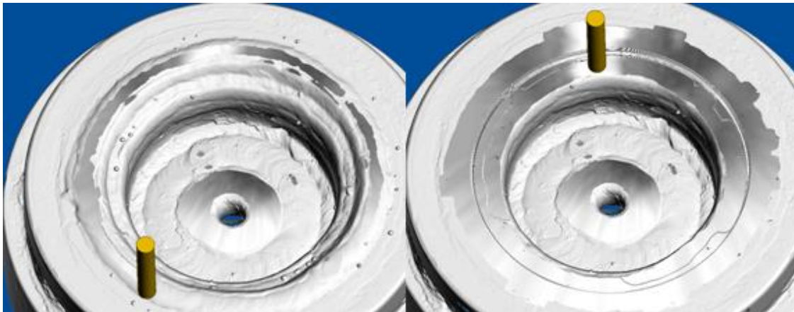
Fig. 4 Simulation of milling process according STL model
