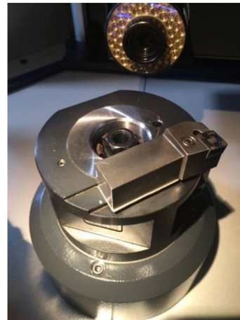
Fig. 4 Cutting insert holder in the measuring device Zoller Genius 3s
