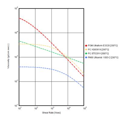
Fig. 2 Graphical representation of the medium viscosity materials
