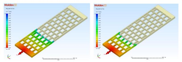
Fig. 9 Status PC XQ83619 in the mold cavity at the end of the injection cycle
