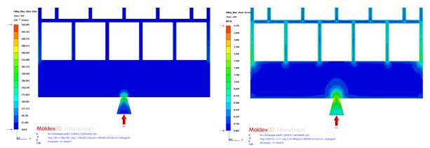
Fig. 5 Shear rate and shear stress in the component cross section of the PC XQ83619 material
