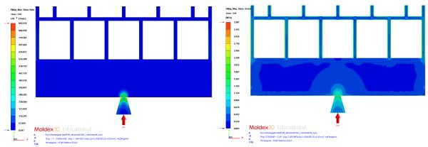
Fig. 6 Shear rate and shear stress in the component cross section of the POM UltramidE3320 material
