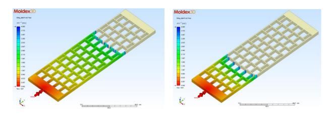
*Fig.* 7 Status PA66 Ultramid 1003-2 in the mould cavity at the end of the injection cycle
