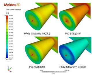
Fig. 11 Temperatures of the inlets at the end of the injection cycle
