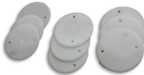
Fig. 1 Polystyrene specimens with 0 %, 0.5 % and 1 % fillers of sodium hydrogen carbonate
