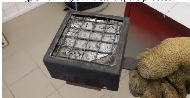
Fig. 10 Specimen after burning
