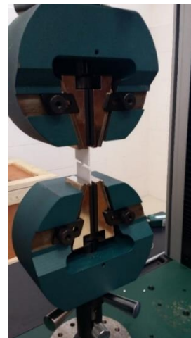
Fig. 3 Specimen after the fracture
