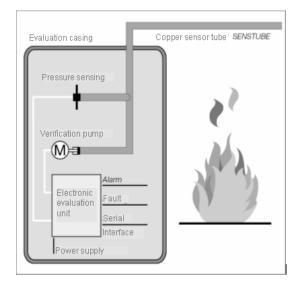
Fig. 3 Principle based on pressure change measurement (1)
