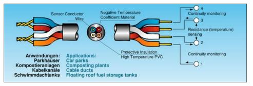
Fig. 2 Analogue cable working on the resistance change principle (1)
