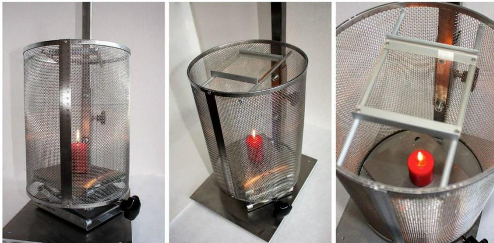
**Fig. 1** Front view of a wire mesh cylinder and a glass plate for determination of soot index of burning candle
