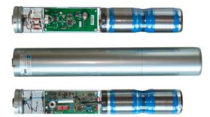
Fig. 4 The RS04 Gamma detector inside and outside view (4)
