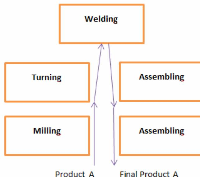
*Fig. 2 One-piece flow manufacturing environment*
