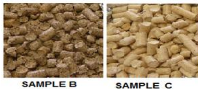
Fig. 1 Sample B – pellets made of softwood with bark, Sample C – pellets made of softwood
