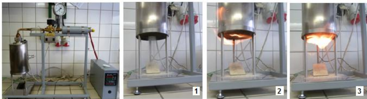
Fig. 6 Ignition time-history of dust clouds when tested according to EN 50281-2-1:2002
