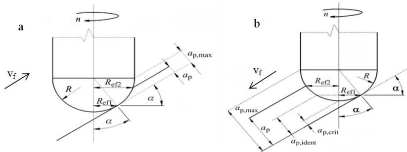
**Fig. 2** (a) Scheme of upward ramping; (b) scheme of downward ramping (9)
