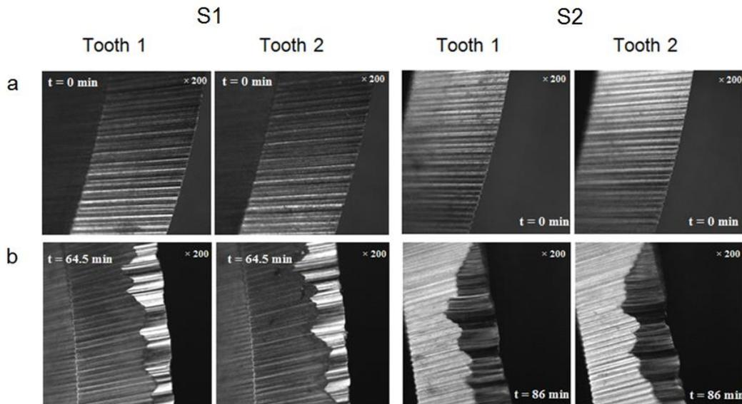
**Fig. 3** (a)Ball nose end mill before cutting,(b)Flank wear after attaining the value of 0.3 mm
