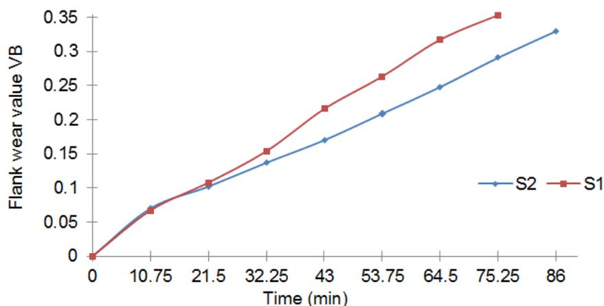
*Fig. 4 The time dependence of flank wear*
