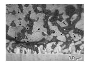
Fig. 2 Cracks propagate through the Sn-rich phase at Sn-Sn grain boundaries after thermomechanical fatigue [3]
