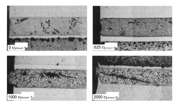
Fig. 1 Heterogeneous coarsening of SnPb40 solder after thermomtchanical fatigue [3]
