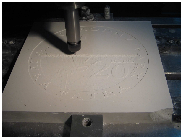
Fig. 3 Machining with raster strategy
