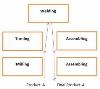
Fig. 2 One-piece flow manufacturing environment
