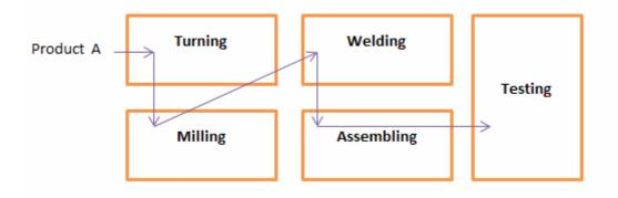
Fig. 1 Batch-and-queue manufacturing environment
