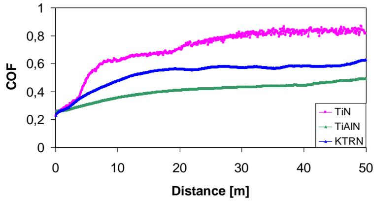
Fig. 5 COF of TiN, TiAlN and KTRN coatings
