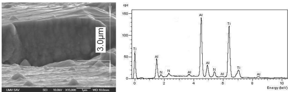
**Fig. 2** Brittle fracture (micrograph) and EDX spectrum of TiAlN coating, thickness 3.0  $\mu\text{m}$
