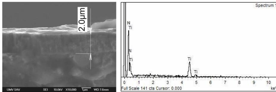
**Fig. 1** Brittle fracture (micrograph) and EDX spectrum of TiN, thickness 2.0  $\mu\text{m}$
