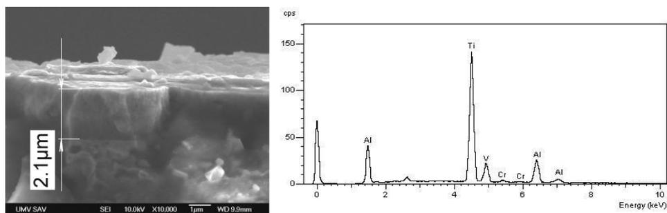
**Fig. 3** Brittle fracture (micrograph) and EDX spectrum of KTRN coating, thickness 2.1  $\mu\text{m}$
