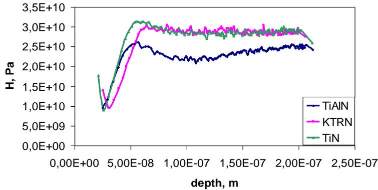
**Fig. 4** The hardness of TiN, TiAlN, and KTRN coatings
