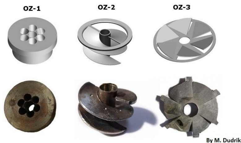
Fig. 3 Design of graphical models of mixers (upper line) and a shot of manufactured mixers (lower line)
