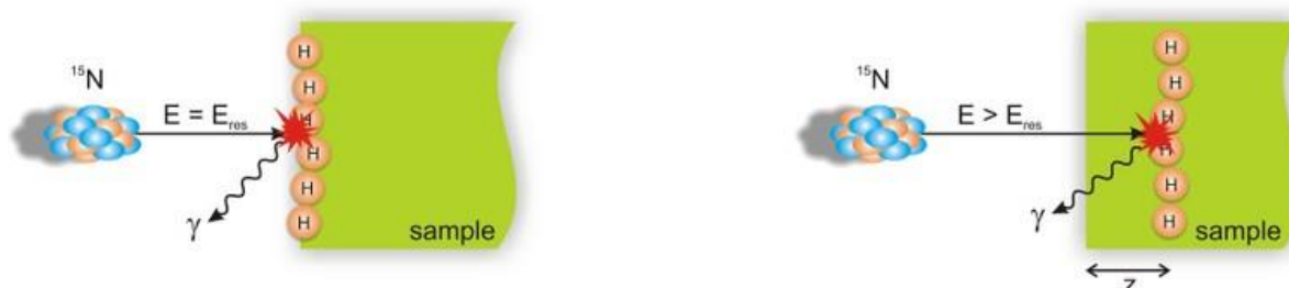
Fig. 6 Principle of hydrogen profiling by NRA with the ^{15}\text{N} ions (8)
