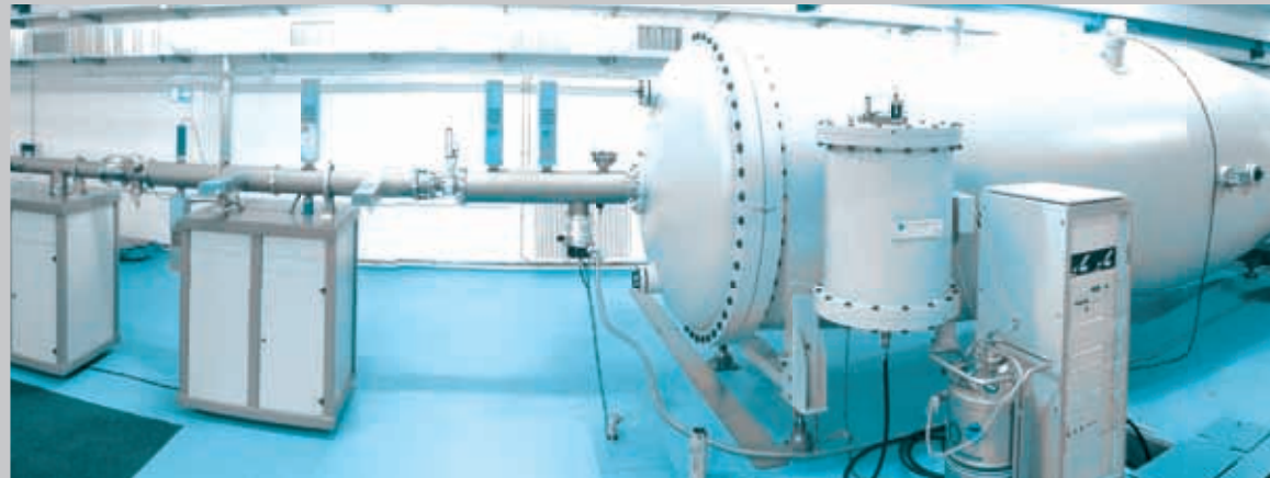
6MV Tandatron used for high-energy ion implantation and irradiation © HZDR Dresden
