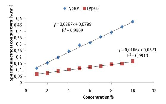
Fig. 5 Dependence of specific electrical conductivity on concentration of emulsion type A and type B at frequency 100kHz On-line monitoring system
