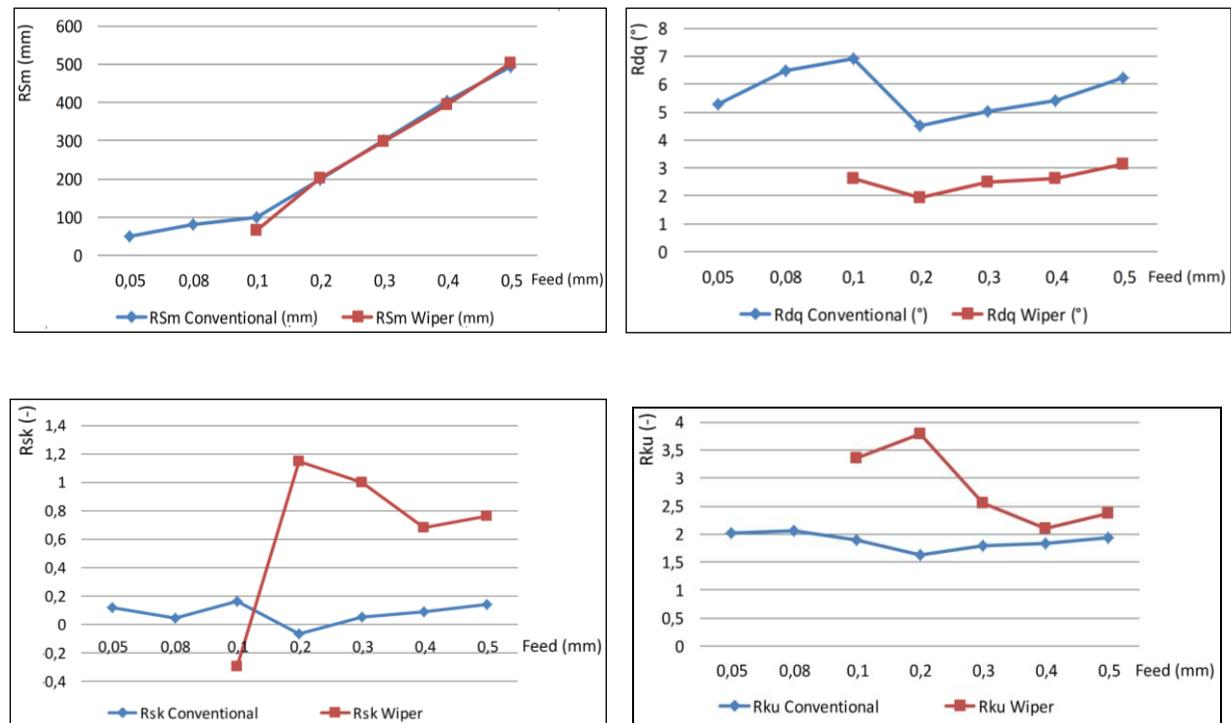
**Fig. 6** Graphs of the surface roughness parameters RSm, Rsk, Rku, Rdq
