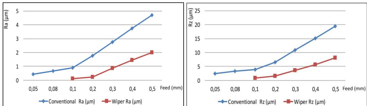
**Fig. 5** Graphs of the surface roughness parameters Ra and Rz
