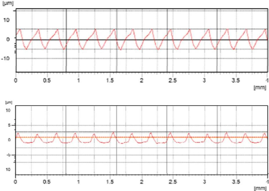
Fig. 4 Roughness profile,  $v_c = 100 \text{ m}\cdot\text{min}^{-1}$ ,  $a_p = 0,25 \text{ mm}$ ,  $f = 0,3 \text{ mm}$ , upper – conventional geometry, lower – wiper geometry
