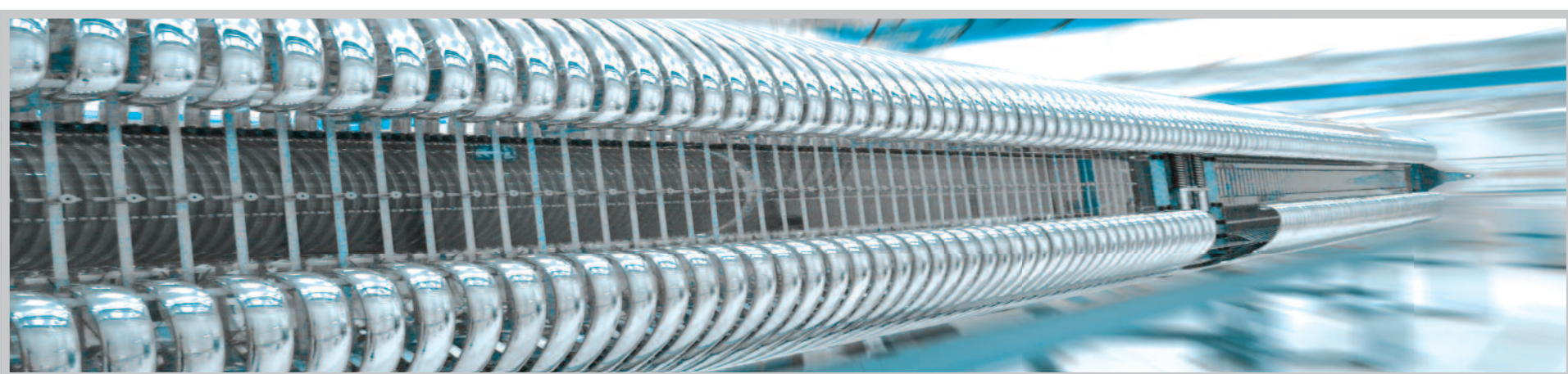
Typical high voltage cascade of an accelerator © HZDR Dresden
