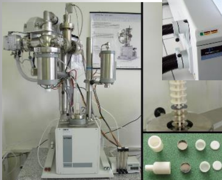
Netzsch STA 409 CD simultaneous thermal analyzer with mass spectrometer (DTA/DSC, TG)
