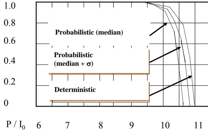
**Fig. 3** Marginal probabilities and median of 81 variants for earthquake occurrence in form of curves of non-exceedance  $R_t(I_o \geq I_{oi})$  of given earthquake size in time interval of 10 000 years in given southern Bohemia site [6, 10]
