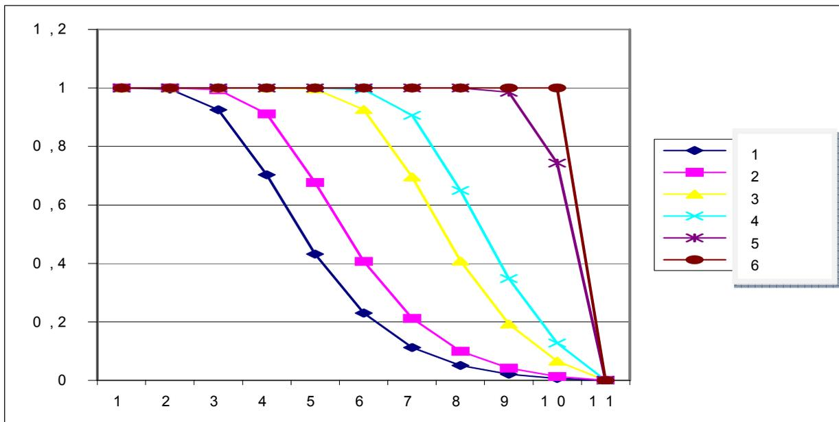
**Fig. 2** Probabilities of earthquake occurrence expressed by curves of non-exceedance  $R_t (I_o \geq I_{\text{oi}})$  in dependence on time interval length for given site.  $P$  – the probability of occurrence of earthquake with intensity  $I_o$  and  $R_t (I_o \geq I_{\text{oi}})$  are probabilities, which mean, that in the time interval  $t$  the value  $I_{\text{oi}}$  will not be exceeded [10];
