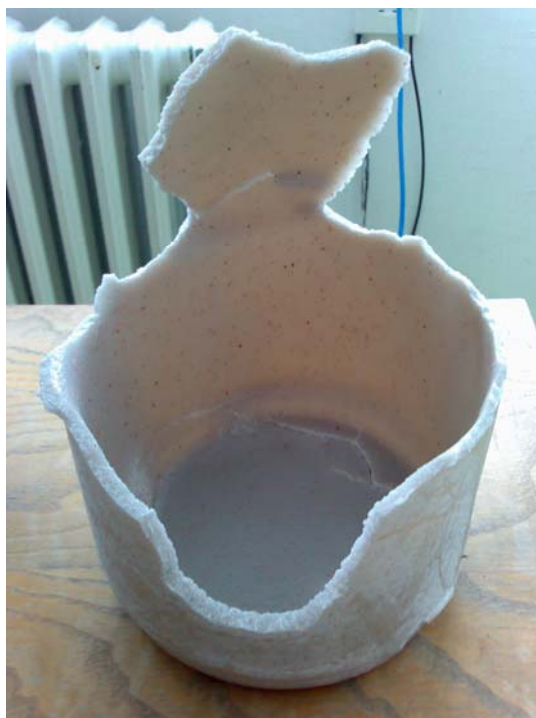
Fig. 5 Deformed shape of the product after de-molding
