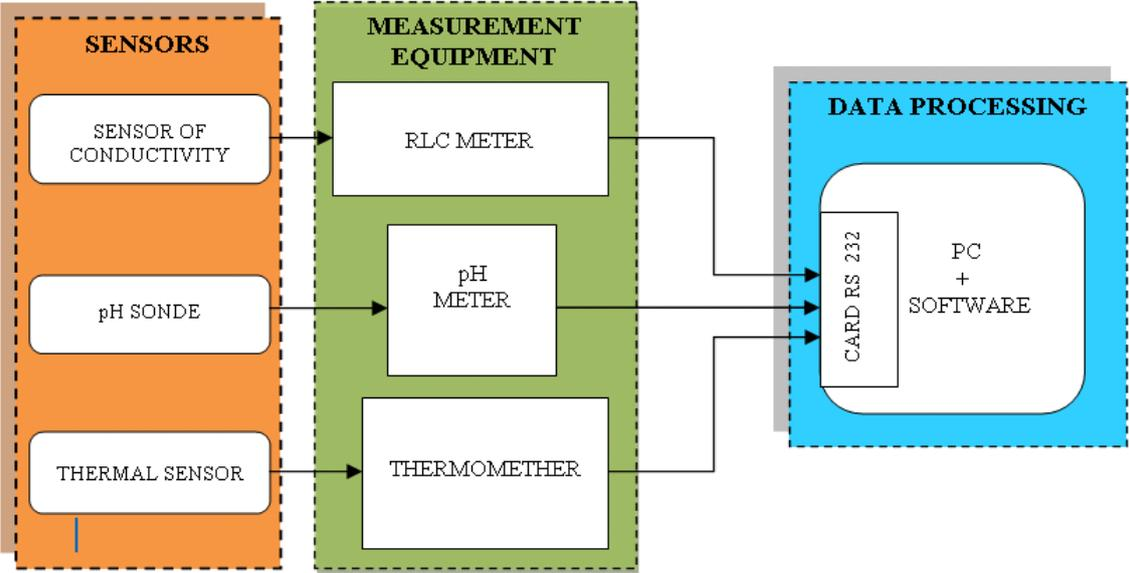
**Fig. 6** The block scheme of the on-line monitoring system
