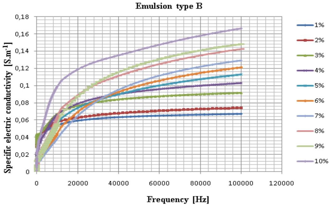
*Fig. 4 Dependence of conductivity on concentration of emulsion type B*
