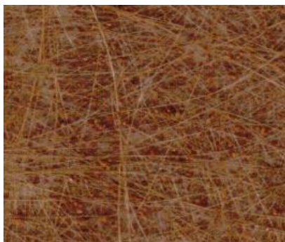
Fig. 3 Red mud (1 g) annealed on the glass wool surface (20 x 20 cm)
