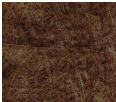
Fig. 4 Black nickel mud (1 g) annealed on the glass wool surface (20 x 20 cm)
