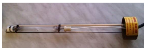
Fig. 5 Medium pressure mercury lamp with output 400 W
