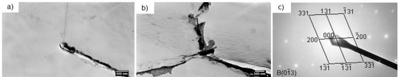
Fig. 2 TEM analysis of grain boundary of AISI 316 a) detail of not sensitized GB, b) detail of sensitized GB (S35), c) diffraction pattern of M_{23}C_6 carbide
