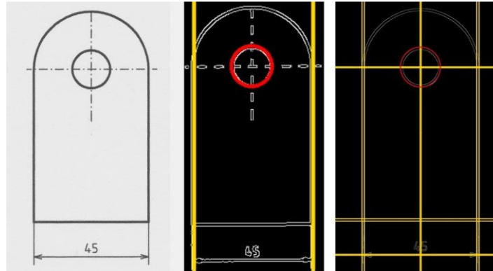
Fig. 8 Hough transform with sample d, results at resolution 150 and 600 DPI
