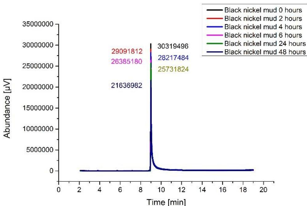
*Fig. 2 Sorption of 3,5-dichlorophenol using black nickel mud*
