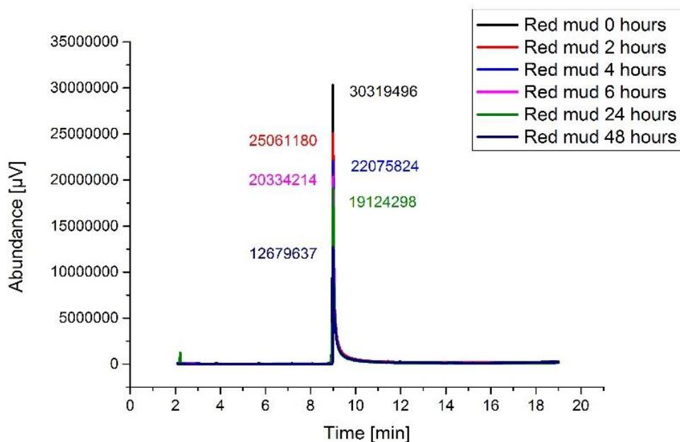
**Fig. 3** Sorption of 3,5 - dichlorophenol using red mud
