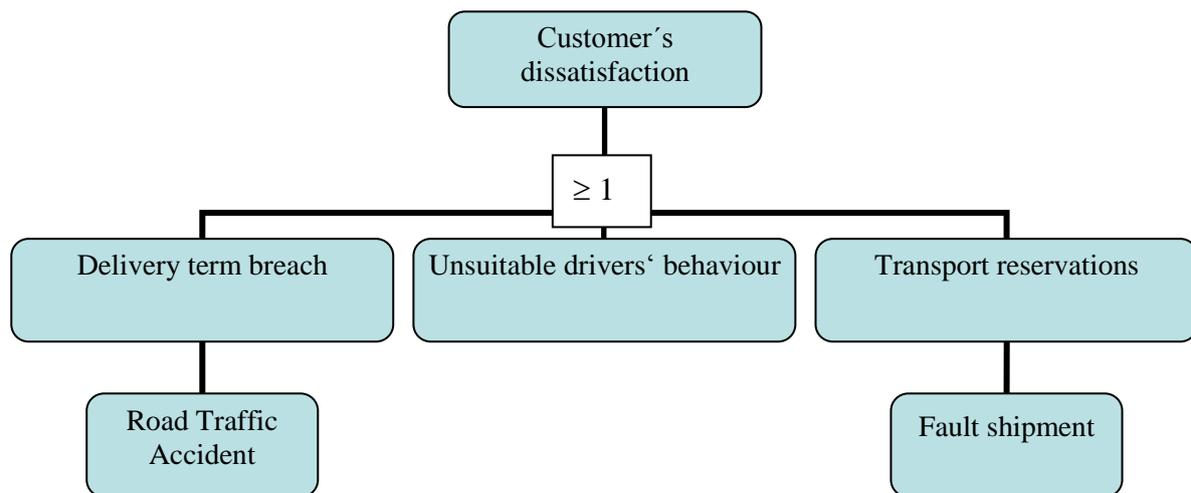
**Fig. 2** Undesired event “Customer’s dissatisfaction” Fault Tree
