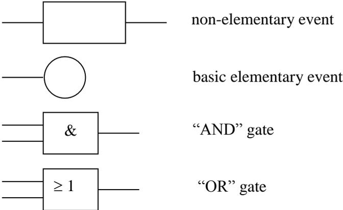
**Fig. 1** Basic graphical symbolism used in the Fault Tree construction
