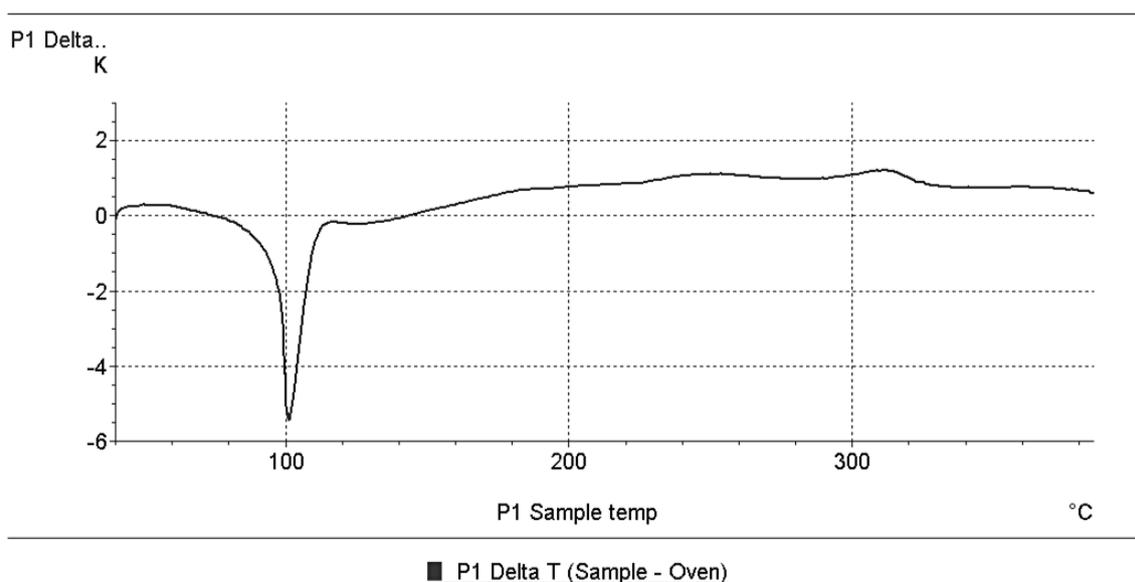
**Fig. 3** DTA at heating rate of 45 °C/h
