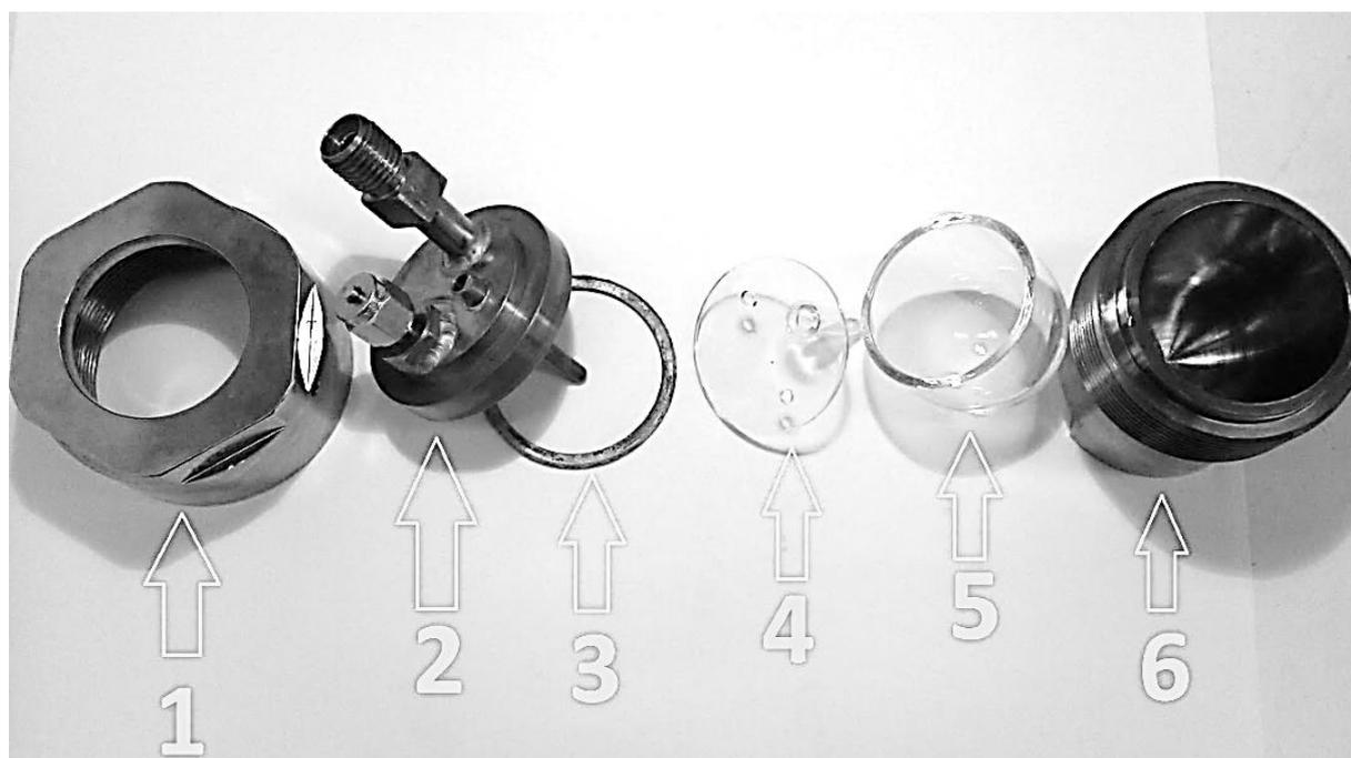
*Fig. 2 SEDEX stainless steel vessel assembly 1 – Top part, 2 – Lid, 3 – Copper o-ring, 4 – Glass liner top, 5 – Glass liner bottom, 6 – Bottom part*
