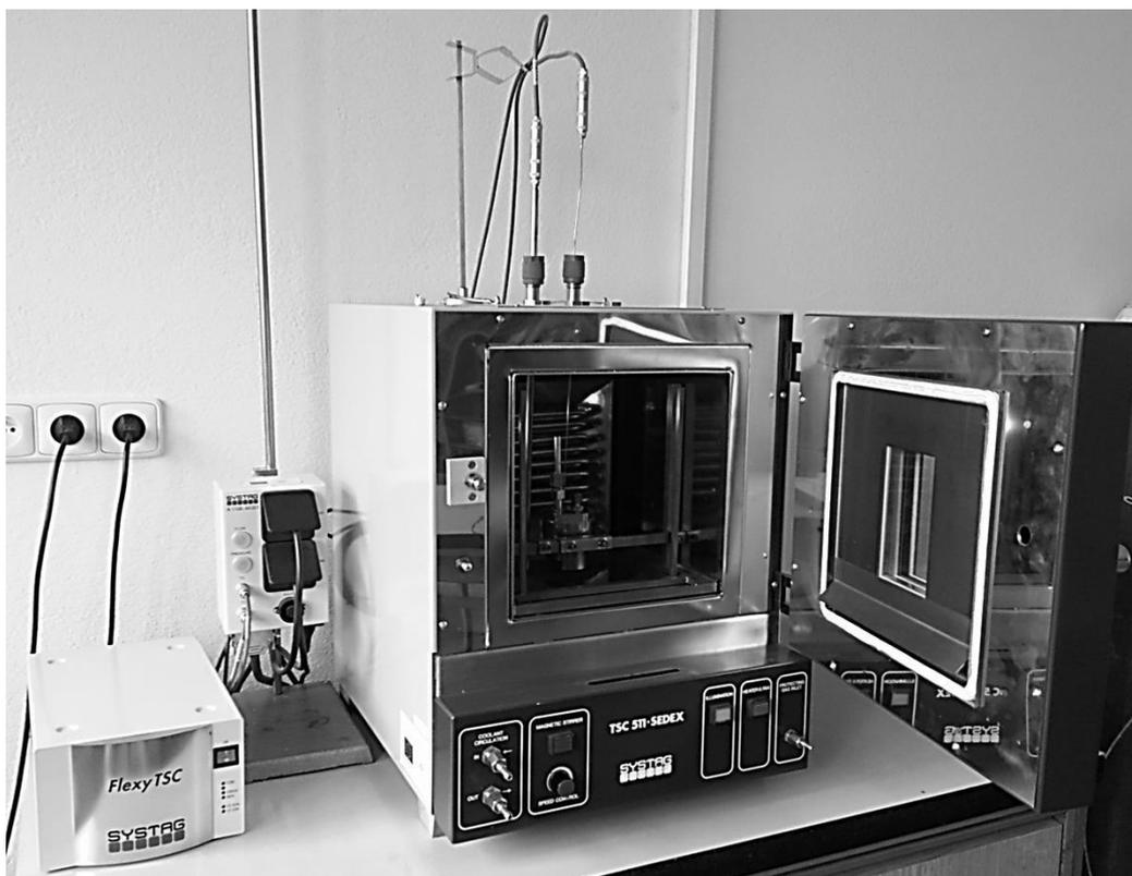
*Fig. 1 SEDEX Safety calorimeter with standard sample vessel*
