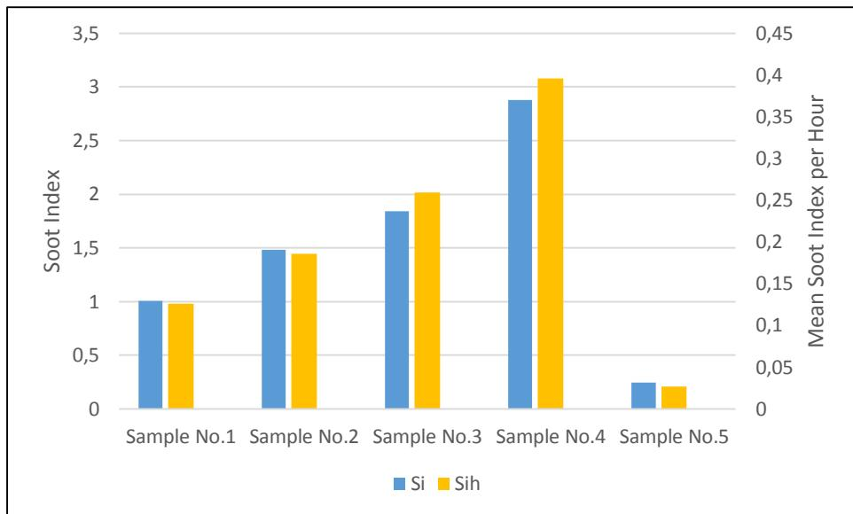
**Fig. 4** Soot index ( $Si$ ), mean soot index per hour ( $Si_h$ ) of candles No.1 – 5
