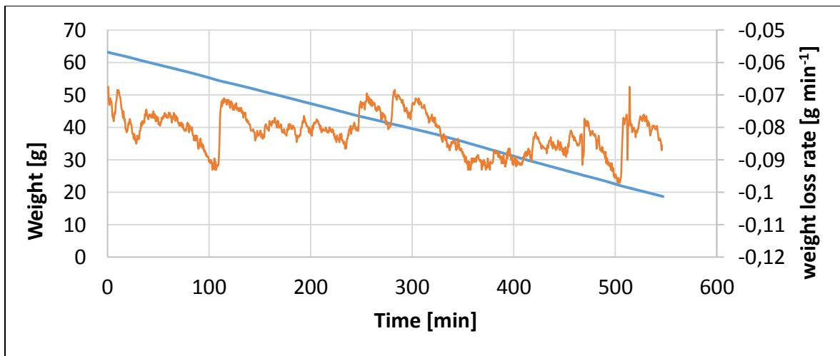
**Fig. 2** Time dependence of weight loss and weight loss rate of burning candle No. 1
