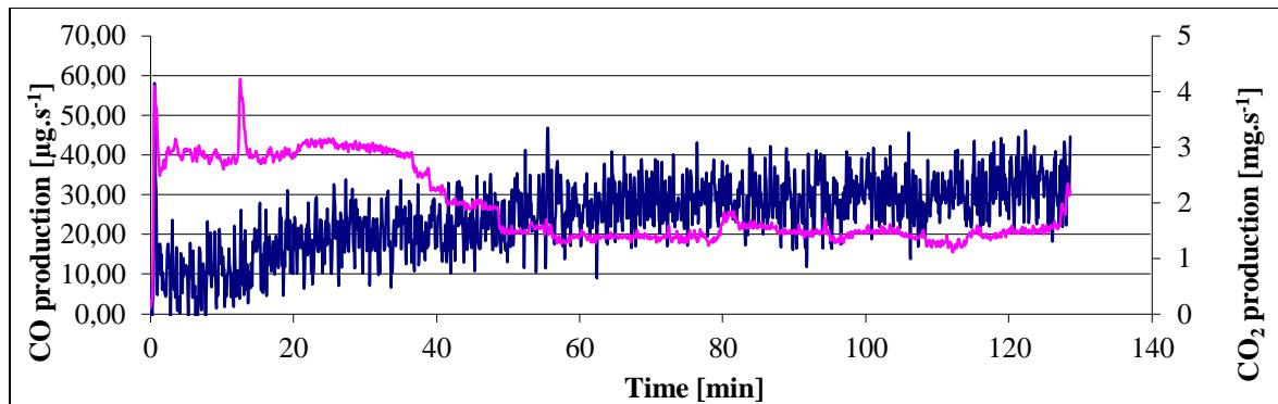
**Fig. 6** Time dependence of the CO and  $\text{CO}_2$  production rate of candle no.1
