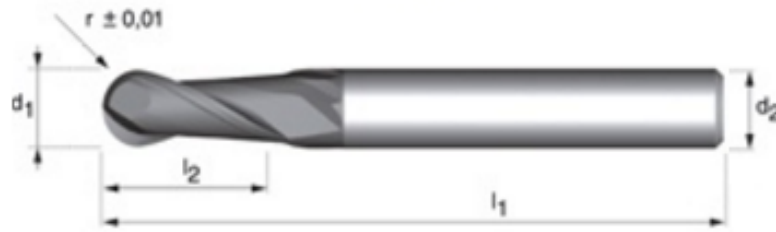
Fig. 3 Cutting tool used in experiments d_1=8 mm, d_2=8 mm, r_1=4 mm, l_2=16 mm, l_1=100 mm.
