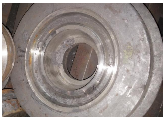
Fig. 1 Die for forge before renovation
