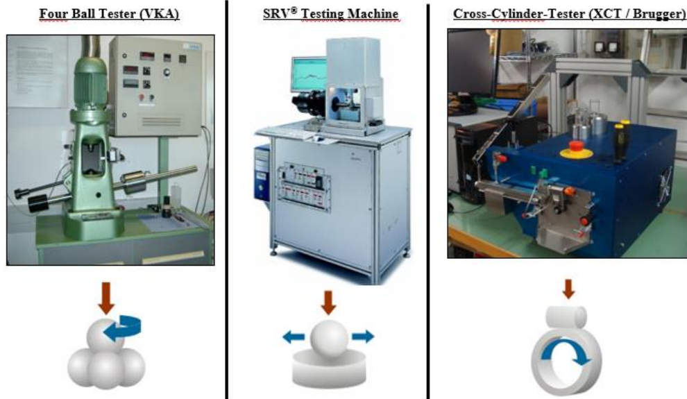
Fig. 2 Test rigs and test specimen configuration
