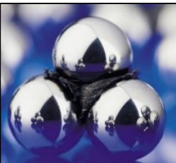
Fig. 6 Welded balls after VKA weld load test
