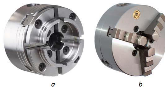
Fig. 2 Segment (a) and common (b) lathe chuck (2)
