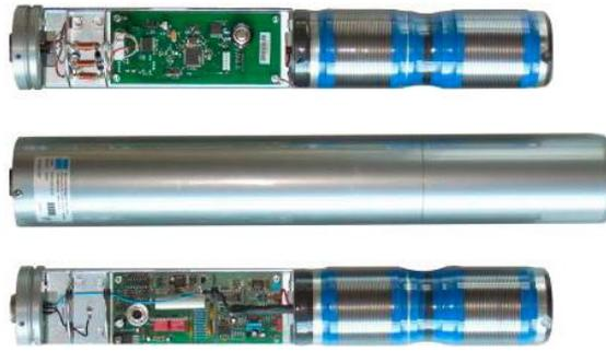
**Fig. 4** The RS04 Gamma detector inside and outside view (4)
