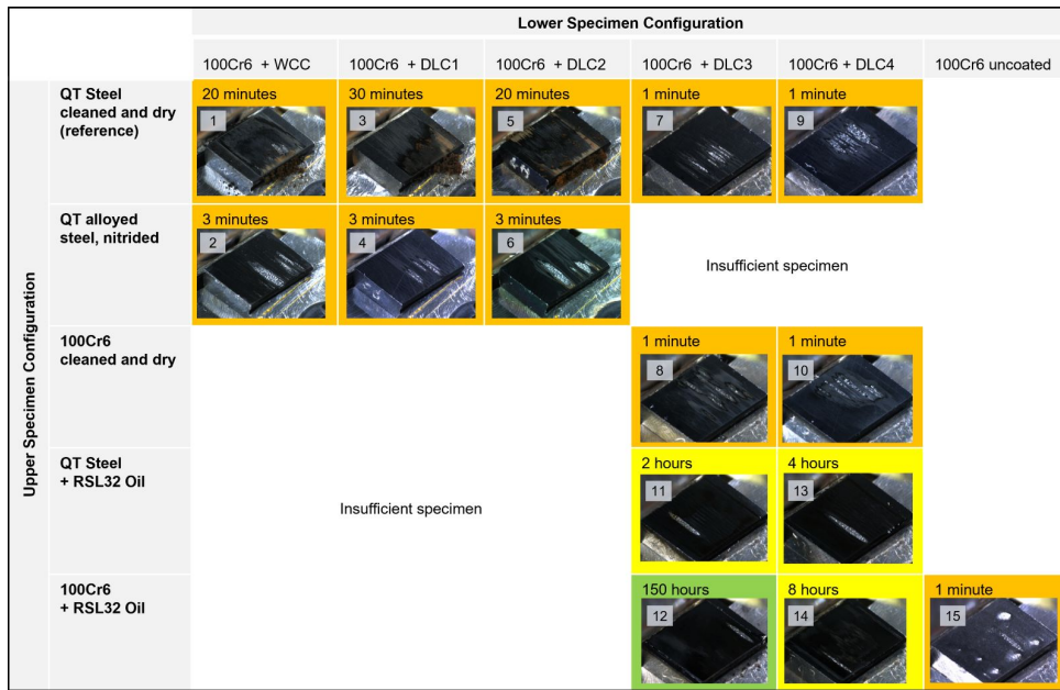
Figure 18: Hard coating screening results as a image table with corresponding run times until damage is visible.
