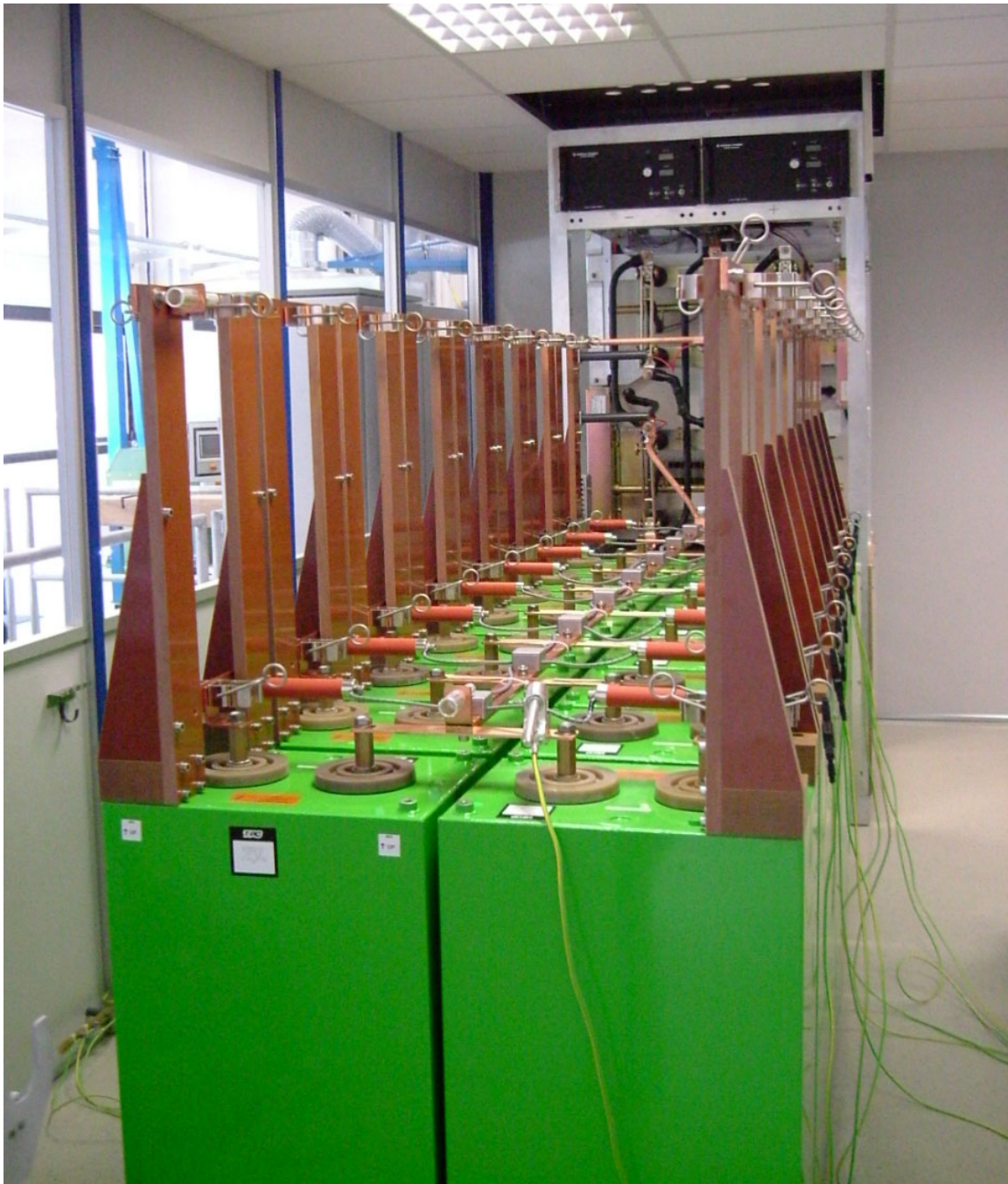
Fig.4 Picture of the 1.44 MJ / 24 kV / 40 kA module which is used in the test facility of pulsed magnetic field coils of the Dresden High Magnetic Field Laboratory.
